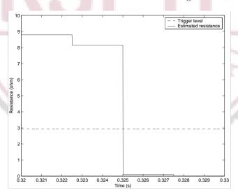
Figure 4: Estimated Resistance during a Fault
