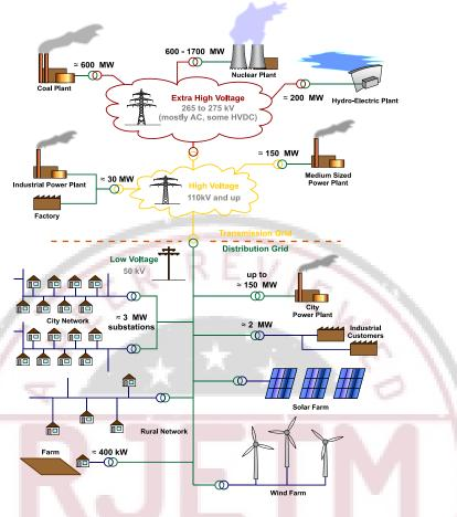
Figure 1: General Layout of Electricity Networks
