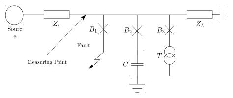
Figure 2: Single Line Diagram for Fault Analysis
